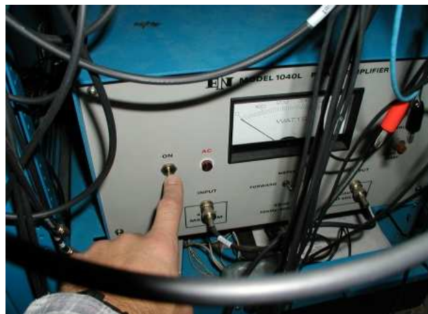
Figure 4.8: Turn off the BNQR RF amplifier
