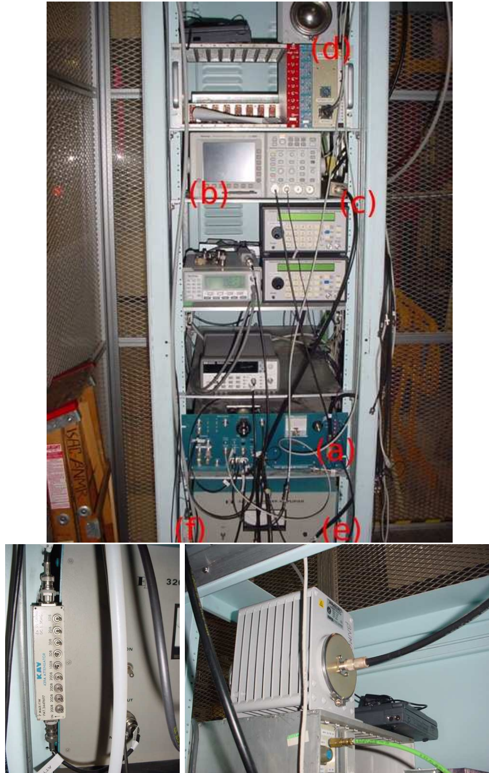
Figure 4.1: (a) Location of the DAC system on platform, (b) Attenuator, and (c) Load.
