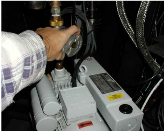
Figure 4.9: Close the valve of the pump for BNQR
