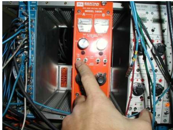
Figure 4.7: Turn off BERTAN HV power supply, it is used to apply a 500V on a ring electrode in the Einzel lens of EL3.
