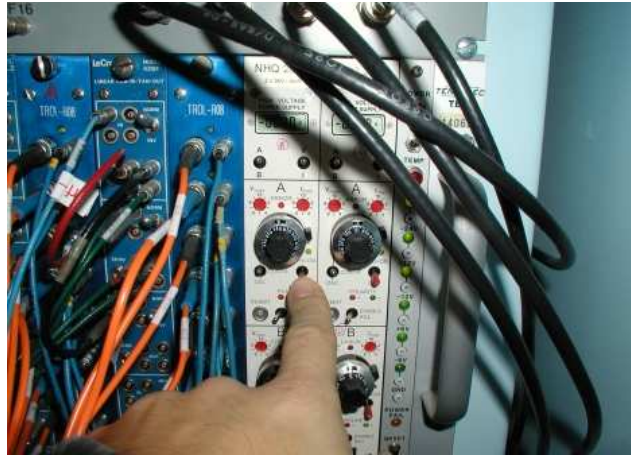
Figure 4.5: Turn off HV of the BNMR Forward detector (A).
