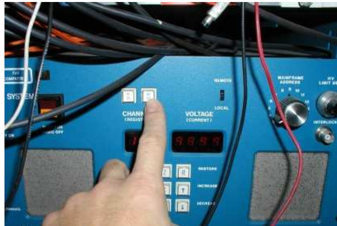
Figure 4.6: Turn off Lecroy HV power system it is for BNMR back detector, BNQR left and right detector. It also powers the neutron beam detector
