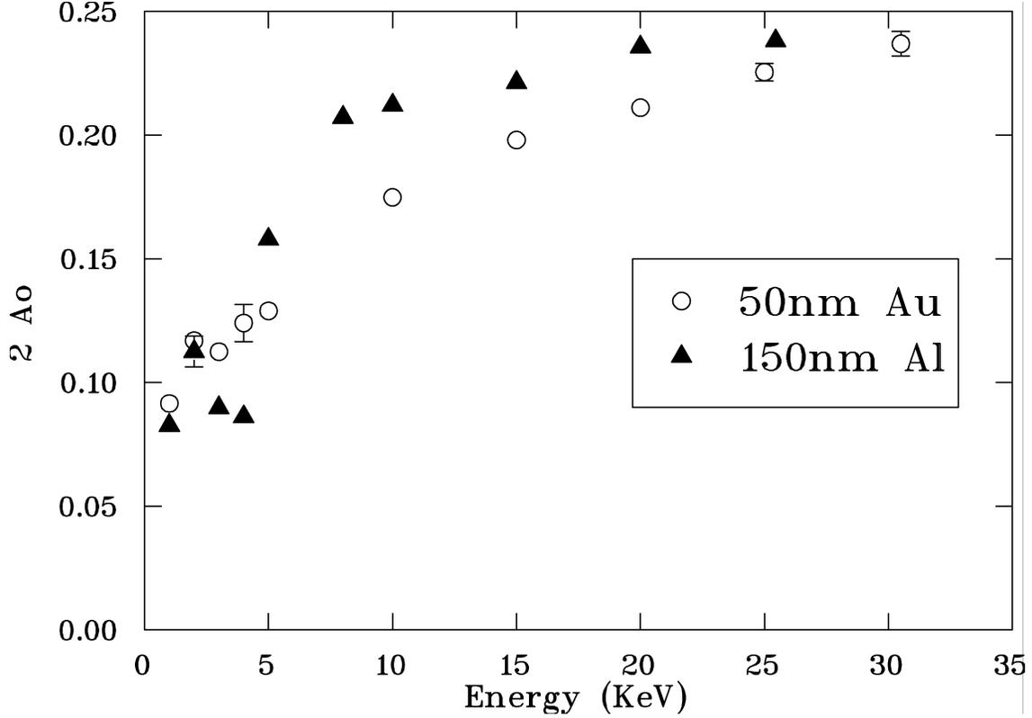
Fig. 3. Total asymmetry ( $2A_0$ ) versus beam energy, for the 50 nm Au sample (circles) and the 150 nm Al sample (filled triangles). Note the drop in total asymmetry at lower beam energies.
