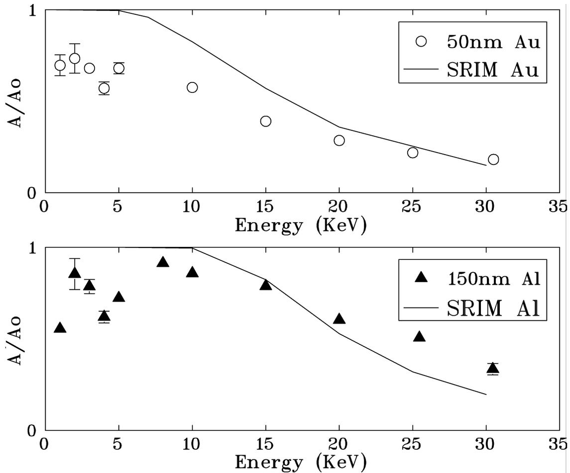
Fig. 4. Top: Normalized amplitude ( $A/A_0$ ) versus beam energy for the 50 nm Au sample (circles). Bottom: Normalized amplitude ( $A/A_0$ ) versus beam energy for the 150 nm Al sample (filled triangles). SRIM predictions are shown for comparison.
