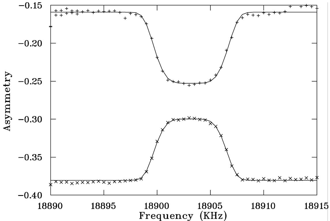
Fig. 2. Spectra in 150 nm Al film on an  $\text{Al}_2\text{O}_3$  substrate, in a 3.0 T magnetic field. Beam energy is 15 KeV. Both spectra are fitted to a modified exponential. The two spectra correspond to “up” and “down” helicities.  $A$  is the resonance amplitude, while  $2A_0$  is the total asymmetry off resonance.
