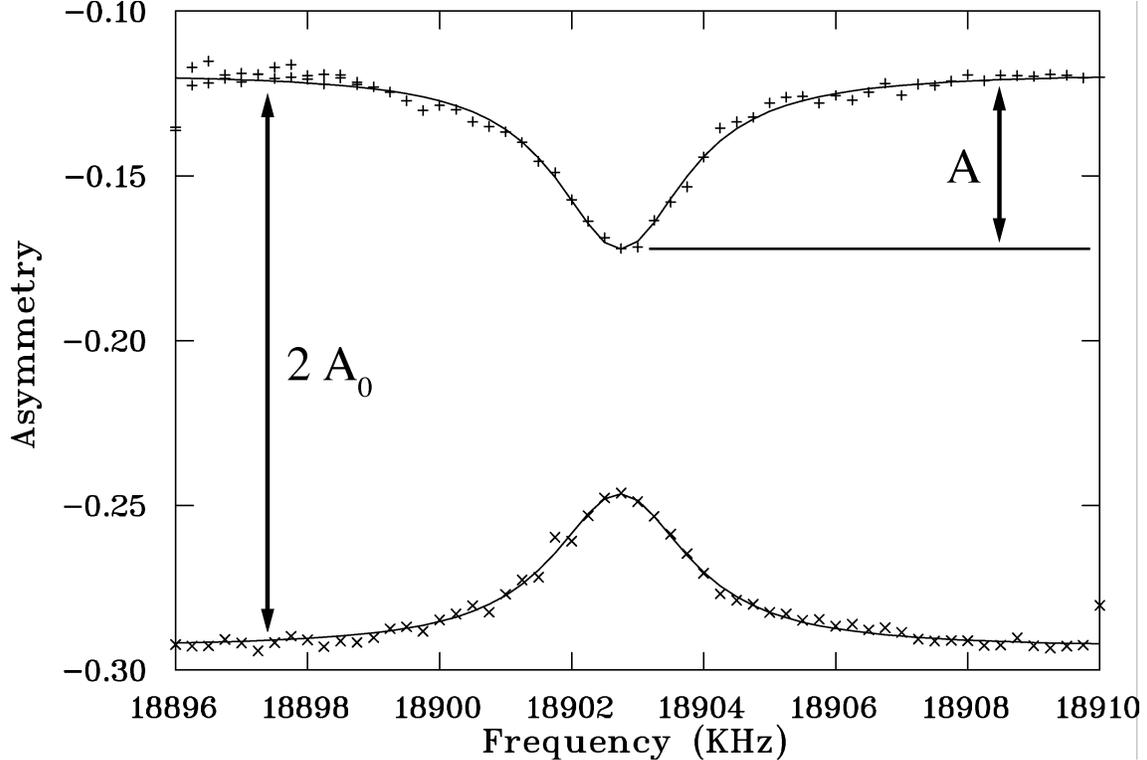
Fig. 1. Spectra in 50 nm Au film on a SrTiO<sub>3</sub> substrate, in a 3.0 T magnetic field. Beam energy is 10 KeV. Both spectra are fitted to a Lorentzian. The two spectra correspond to “up” and “down” helicities.  $A$  is the resonance amplitude, while  $2A_0$  is the total asymmetry off resonance.
