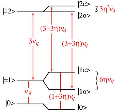
FIG. 4. The energy levels for  $\mathcal{H}_q/h$  (left-hand side) and  $(\mathcal{H}_q + \mathcal{H}_\eta)/h$  (right-hand side). The possible transitions induced by an oscillating field  $B_1$  are also indicated.
