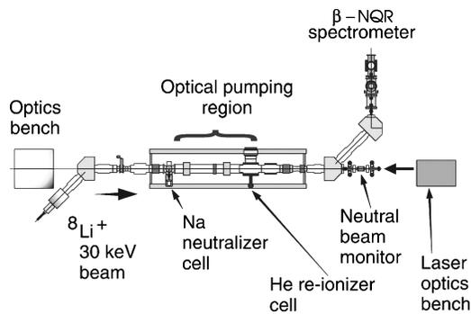
FIG. 1. A schematic of the experimental layout. The 30 keV  $^8\text{Li}^+$  ion beam is neutralized in the Na cell and then reionized in the He cell. In between, the beam is optically pumped with a laser tuned to the D1 optical transition of the  $^8\text{Li}$  atom. The resulting polarized ion beam is guided to the  $\beta$ -NQR spectrometer.
