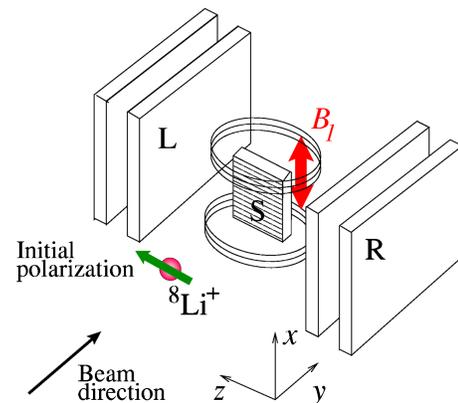
FIG. 3. A schematic of the spectrometer for  $\beta$ -detected nuclear quadrupole resonance. The spin polarization is perpendicular to the beam direction and the oscillating  $B_1$  magnetic field. The principal axis of the electric field gradient at the Li stopping site must have a component along  $\hat{z}$  in order for a signal to be detected at zero applied field.
