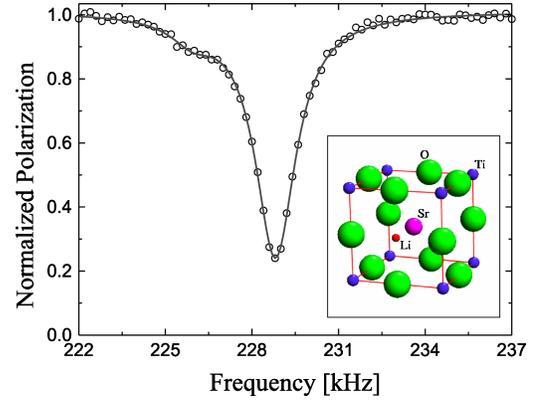
FIG. 5. The  $\beta$ -NQR spectrum obtained for a  $\text{SrTiO}_3$  single crystal at room temperature and zero external field. Inset: The cubic unit cell of  $\text{SrTiO}_3$  showing the proposed interstitial Li site at the face center.
